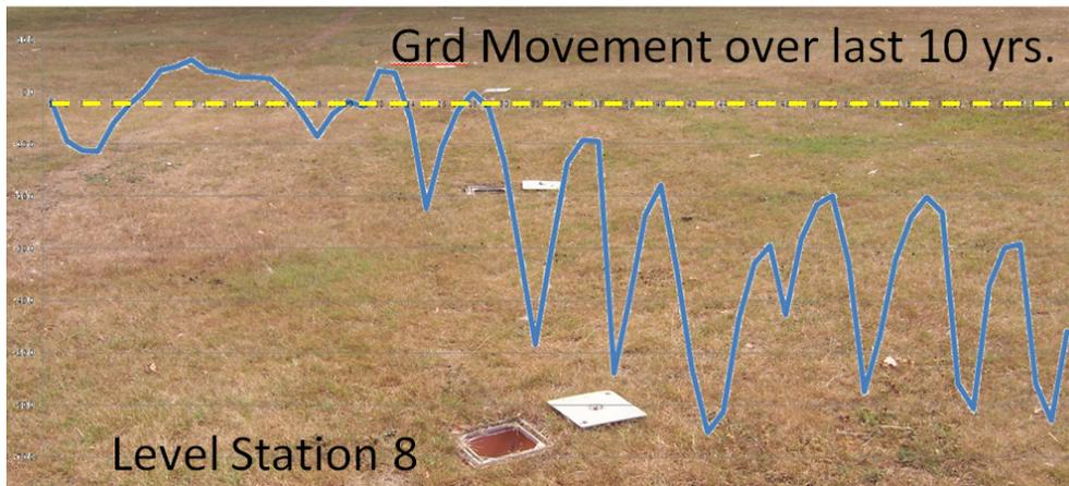
*The blue line plots ground movement at Station 8 (galvanised cover removed to take reading) since 25th May, 2006, which was a 'mini-surge year' delivering around 48,000 claims. Although some modest rehydration took place in the winter of 2006, the general trend has been downwards since.*
